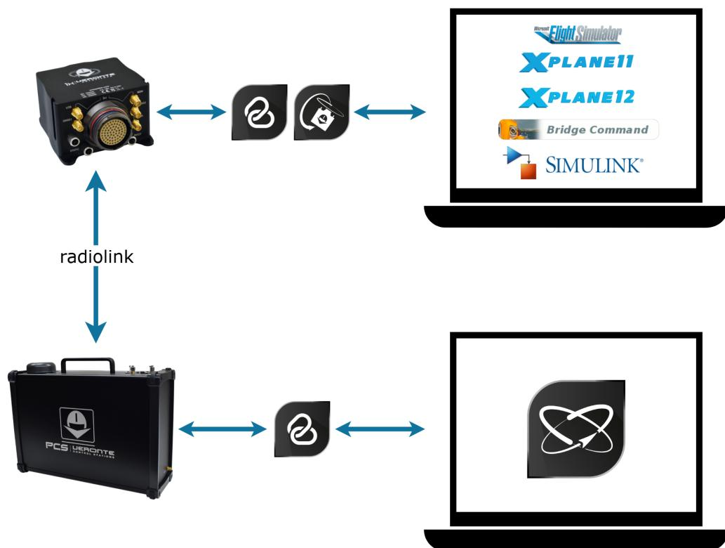
**HIL with radiolink diagram**
